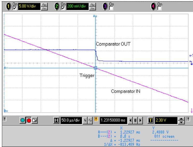
**Figure 7-1. Transfer Characteristic of Digital CMOS Input with Linearly Decreasing Input Voltage**
