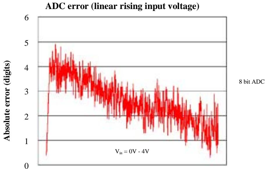
**Figure 7-8. Absolute Error of 8 Bit Sigma Delta DAC in Digits (LSB)**
