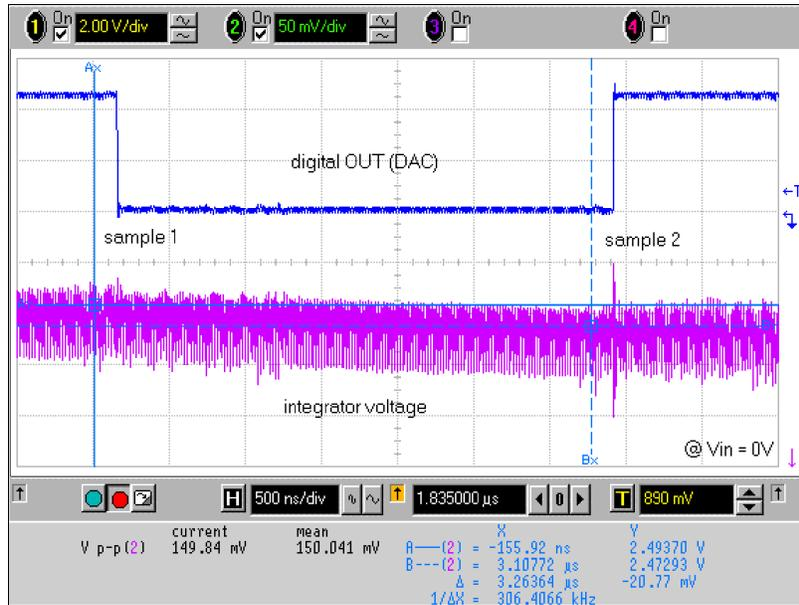
Figure 7-7. Integrator Voltage at 306 KHz Sampling Frequency
