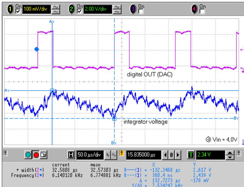
**Figure 7-6. Integrator Voltage at 30.6 KHz Sampling Frequency**
