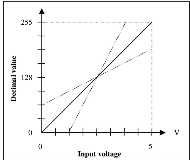
Figure 3-9. Continuous Line Shows the Ideal Linear ADC Transfer Characteristic
