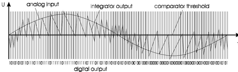
**Figure 3-4. Signals in a First Order Sigma Delta Modulator**
