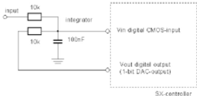
**Figure 4-2. Simple Implementation of a First Order Sigma Delta-Modulator**
