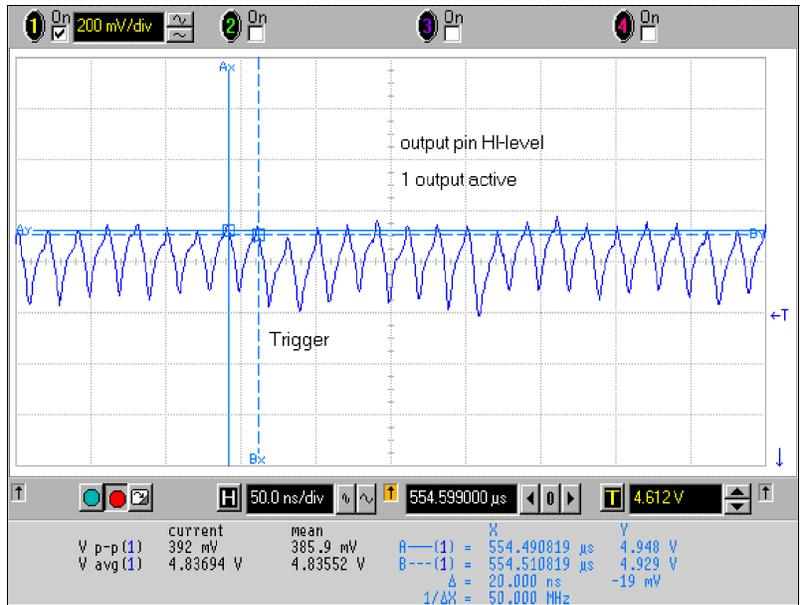
Figure 7-4. Output Voltage at High Level
