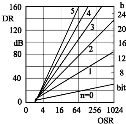
Figure 3-5. Dynamic Range of a Sigma Delta Modulator
