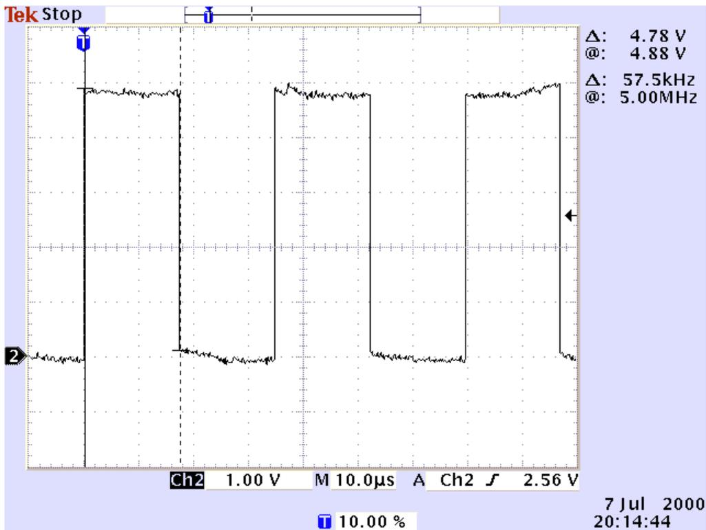
Figure 5-7. Output Signal from ADC at  $V_{in} = \frac{1}{2} V_{DD}$
