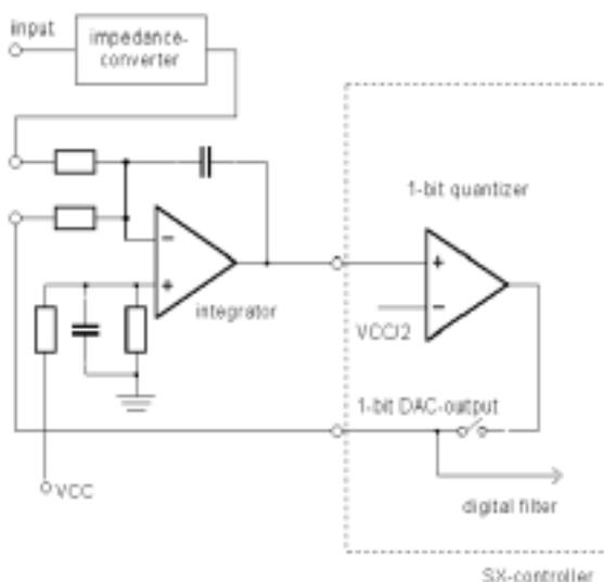
**Figure 4-1. Implementation of a First Order Sigma Delta Modulator with Operational Amplifier**
