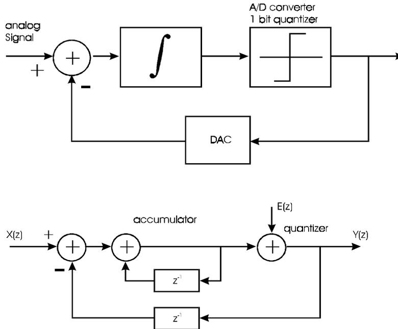
**Figure 3-2. Principle of Sigma Delta Modulation a) Building Blocks b) Time Discrete Representation**
