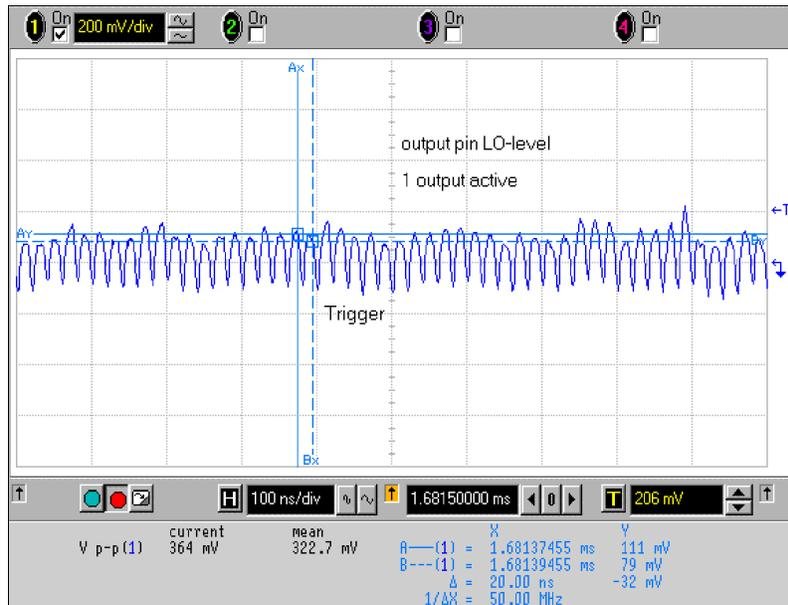
**Figure 7-5. Output Voltage Low Level**
