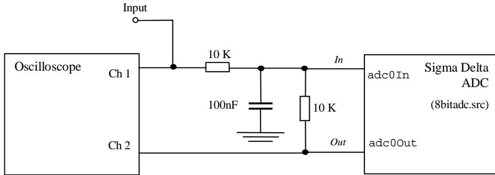
Figure 5-2. Overview of the Test Environment
