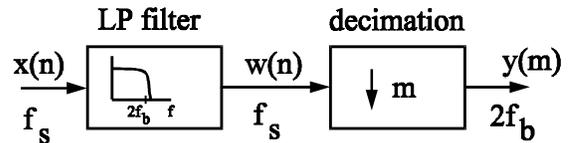
Figure 3-6. Digital Portion of a Sigma Delta Converter
