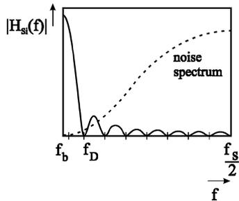
Figure 3-7. Frequency Response of Si-Function
