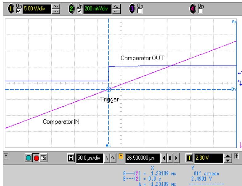
**Figure 7-2. Transfer Characteristic of Digital CMOS Inputs with Linearly Increasing Input Voltage**
