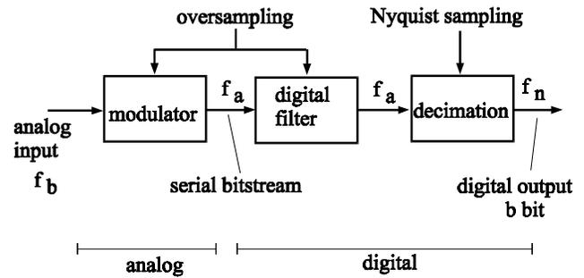
Figure 3-1. Building Blocks of a Sigma Delta Converter
