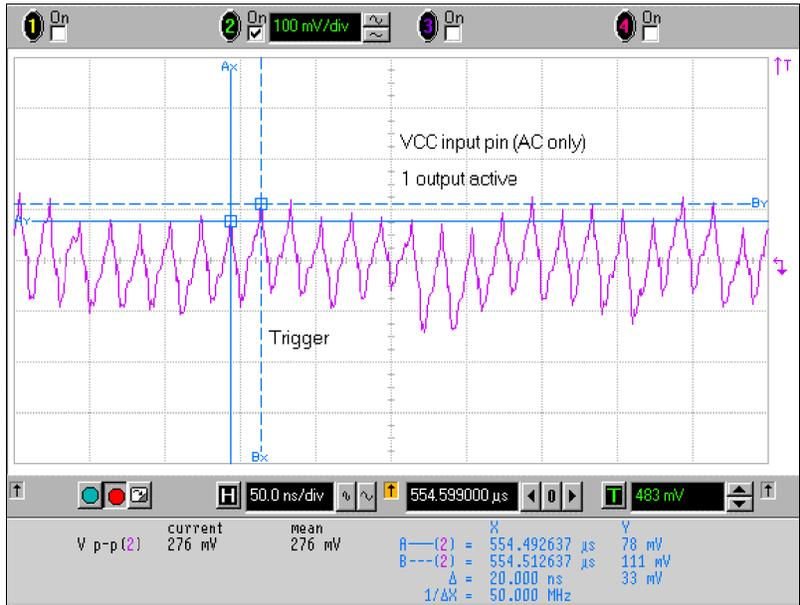
Figure 7-3. Voltage Bounce at  $V_{DD}$  Pin
