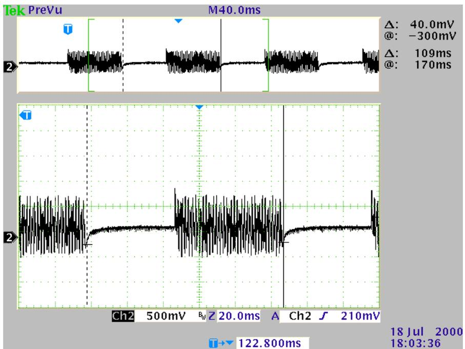
Figure 9-11. Cycle Time Measured to 109ms
