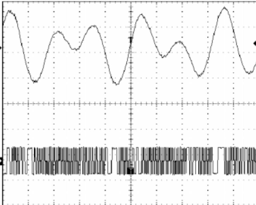
Figure 4-1. PWM Signal (lower part) and Filtered DTMF Output (upper part) for '1' (#1)
