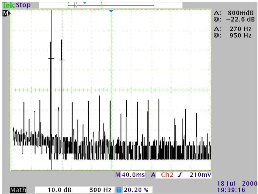
Figure 9-6. The '\*' Digit (star) with  $f_L=946\text{Hz}$  and  $f_H=1216\text{Hz}$ . Level Difference to Nearest Noise Component is 26dB ( $f=2.16\text{kHz}$ ).
