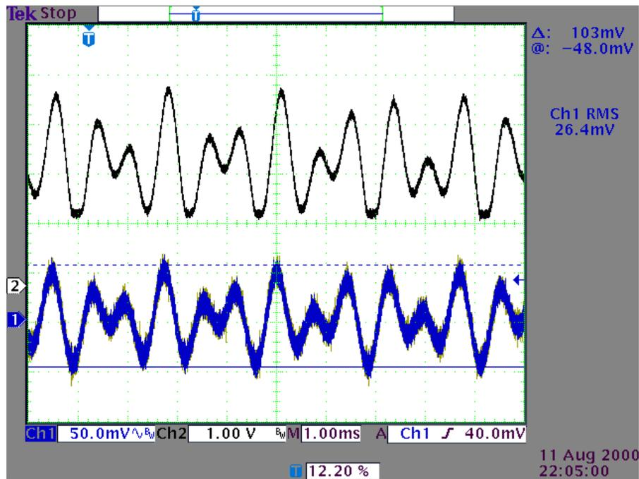
Figure 7-3. Input Signal (ch1) = 102mV p-p When the Input Signal to the A/D (ch2) Starts Clipping
