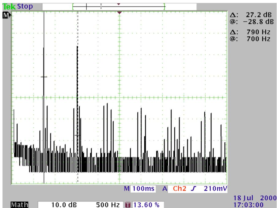
Figure 9-3. The '3' Digit with  $f_L=701\text{Hz}$  and  $f_H=1486\text{Hz}$ . Level Difference to Nearest Noise Component is 26dB ( $f=2.19\text{kHz}$ )
