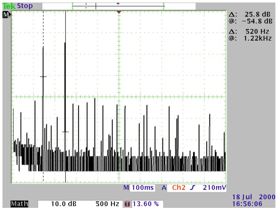
Figure 9-1. The '1' Digit with  $f_L=701\text{Hz}$  and  $f_H=1216\text{Hz}$ . Level Difference to Nearest Noise Component is 24dB ( $f=1.9\text{kHz}$ )
