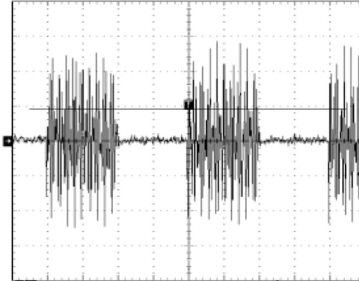
**Figure 4-2. DTMF Output (when dialing a sequence of numbers and special characters)**
