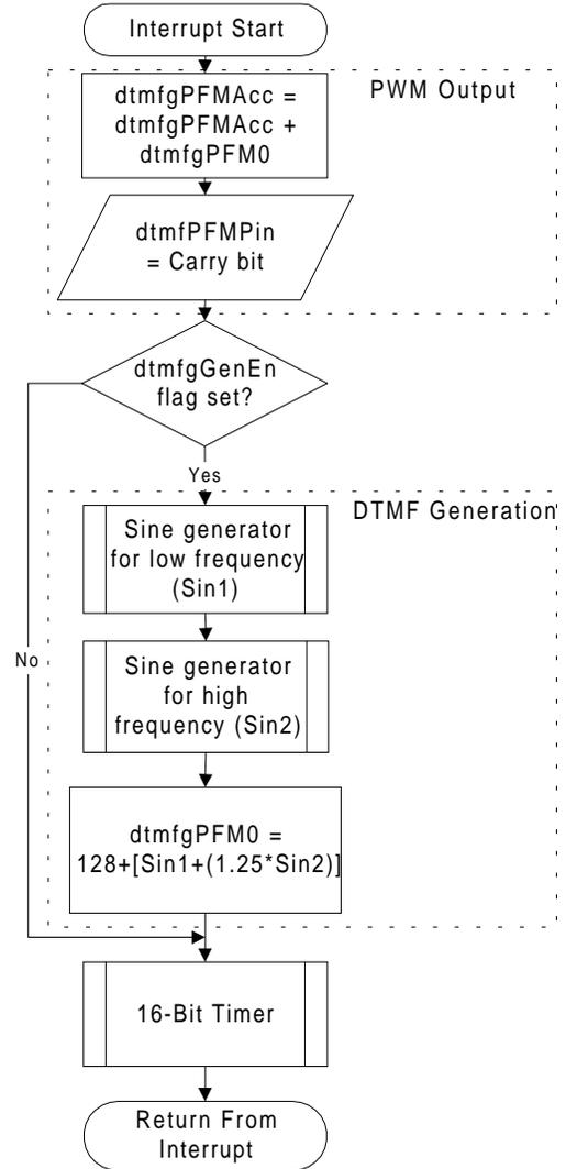
**Figure 4-4. Interrupt Service Routine Used in DTMF Generation**
