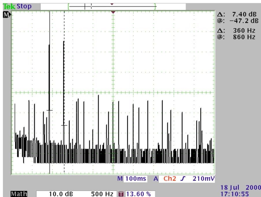
Figure 9-5. The '7' Digit with  $f_L=857\text{Hz}$  and  $f_H=1217\text{Hz}$ . Level Difference to Nearest Noise Component is 26dB ( $f=2.07\text{kHz}$ )
