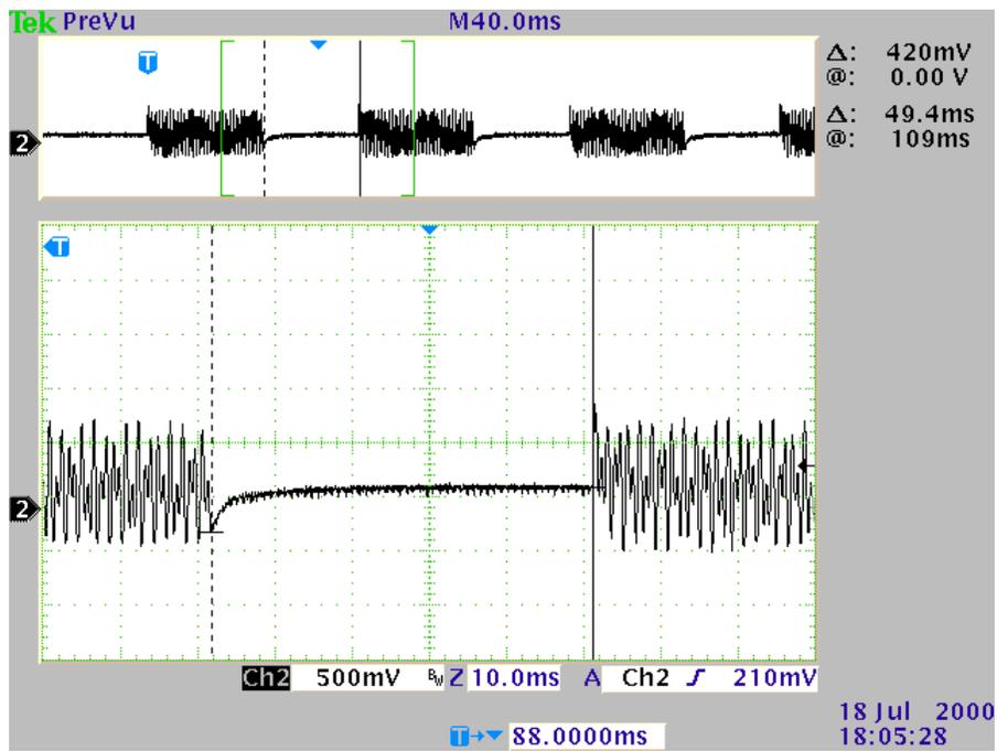
Figure 9-10. Inter-Digit Interval Measured to Approximately 50ms
