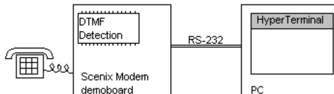
Figure 7-2. DTMP Detection
