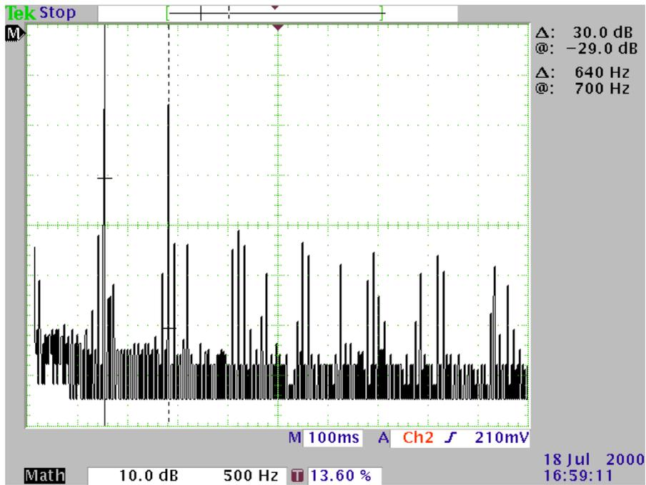
Figure 9-2. The '2' Digit with  $f_L=701\text{Hz}$  and  $f_H=1344\text{Hz}$ . Level Difference to Nearest Noise |Component is 24dB ( $f=2.05\text{kHz}$ )
