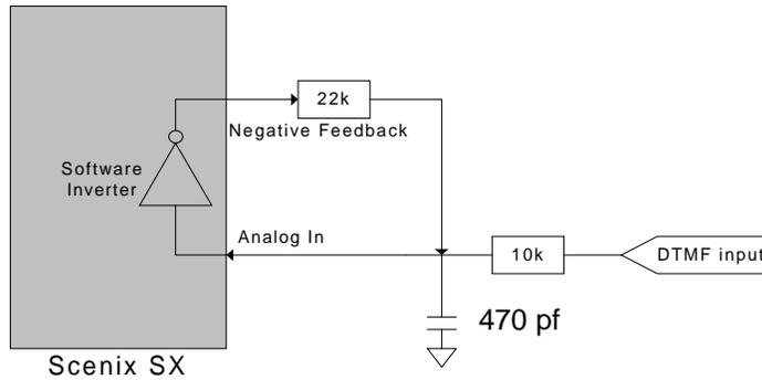
**Figure 4-7. Software Sigma Delta A/D Converter**
