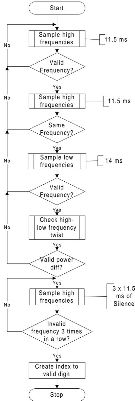
**Figure 4-11. Flowchart of the dtmfGetValid Subroutine**
