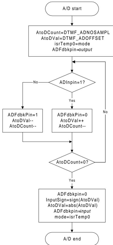
**Figure 4-8. A/D Sample Routine in Interrupt**
