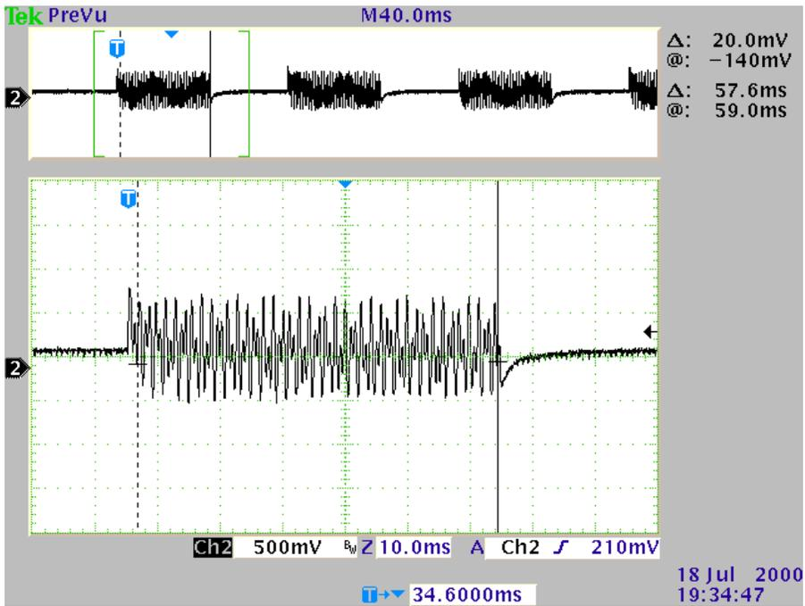
Figure 9-7. Signal Duration Measured to 58ms
