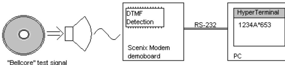
Figure 7-5. Testing DTMF Detection According to Bellcore Specification
