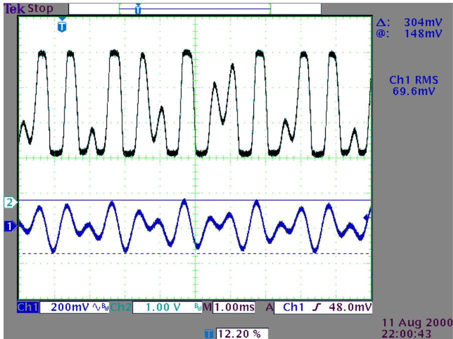
**Figure 7-4. Input Signal (ch1)= 300mV p-p Results in a Clipped Signal to the A/D (ch2)**
