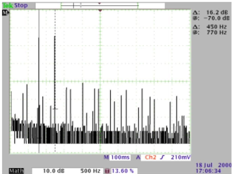
Figure 9-4. The '4' Digit with  $f_L=775\text{Hz}$  and  $f_H=1217\text{Hz}$ . Level Difference to Nearest Noise Component is 25dB ( $f=1.99\text{kHz}$ )
