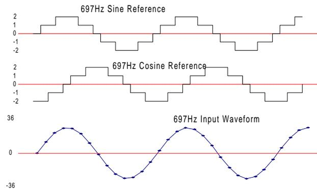
**Figure 4-5. Reference Wave Comparison with Input Signal**
